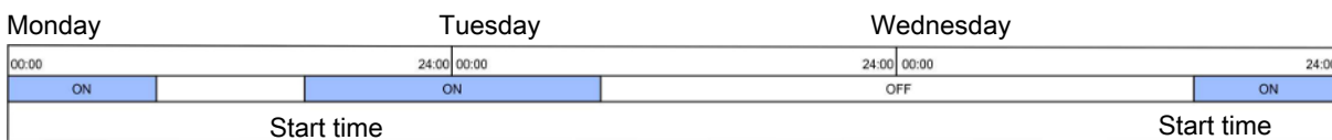
Figure 25: If an ON-time runs past midnight on a day when the 24-hour clock is not active, the function will remain ON until the time has elapsed.
